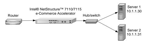
Figure 4-2: Single 7110/7115, Multiple Server Installation
